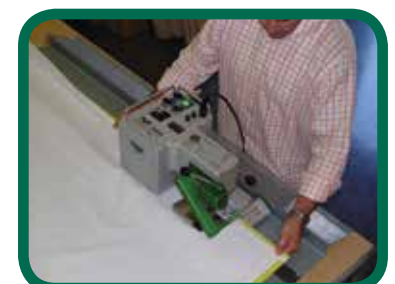
Track/Table Flat Hem Weld, USA
