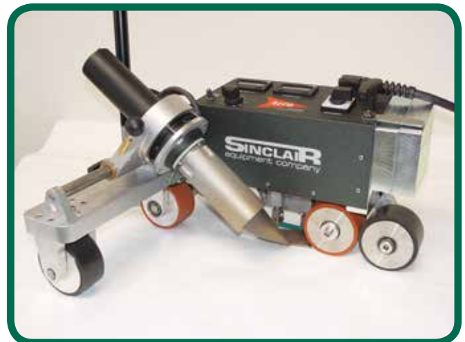
Aero Overlap Welder
